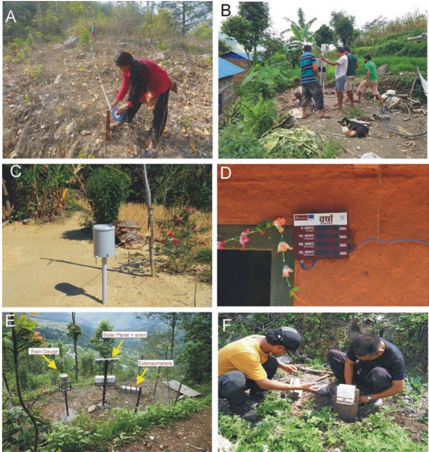
Fig. 20.6 Some examples of landslide early warning systems in Nepal. (a) Measuring landslide displacement by moving peg method; (b) LEWS installation in Bijulikot, Ramechhap (Source: Shreelal Poudel); (c and d) automatic rain gauge and rainfall display board in Kailali; (e) LEWS in Sundrawati village, Dolakha; (f) LEWS installation in the Khani Gau, Gorkha. (Source: Lulu Sinjali)
