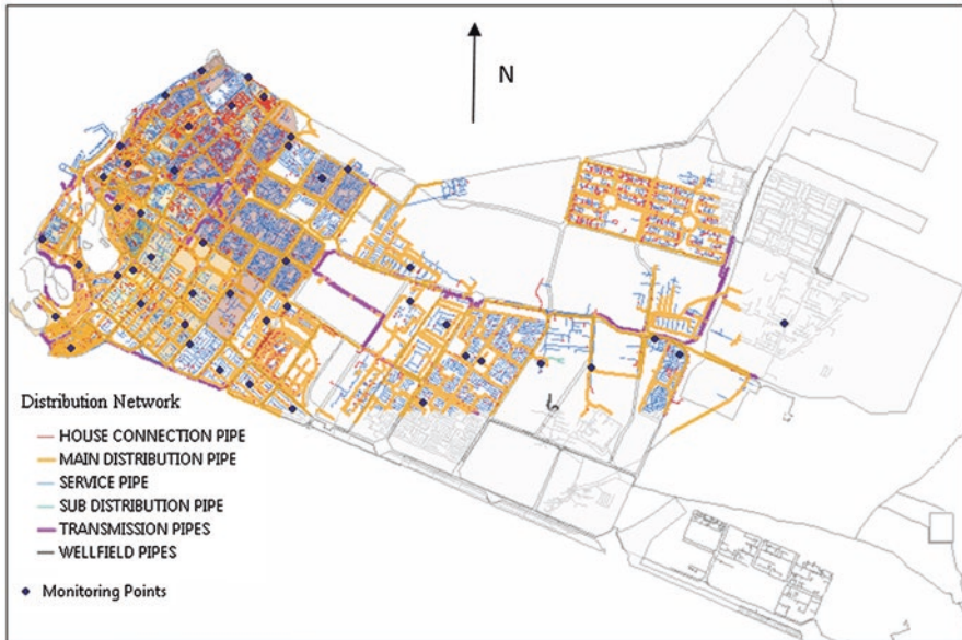
Fig. 15.5 Water distribution network of SEWA (drawn not to scale). Note: The position of the circle represents the sustainability-resilience index. Scenario numbers are shown in circle. (Adapted from Mortula et al. (2019))
