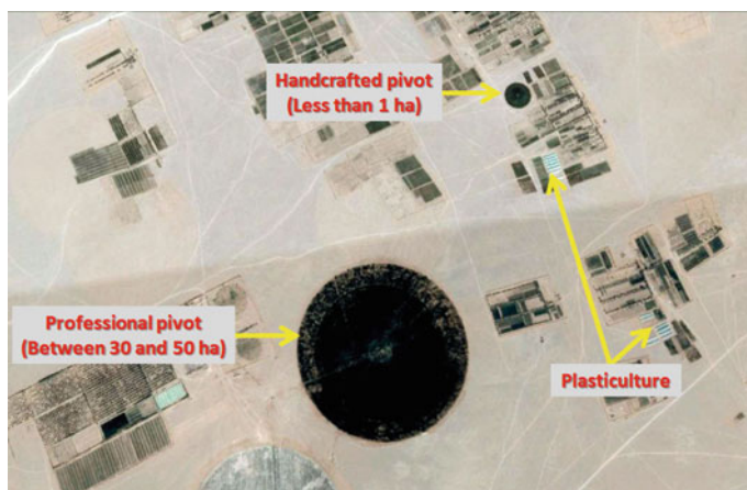
Fig. 1 Size of the pivots used in the irrigated perimeters of Aougrou. Source Image Google Earth, 2016
