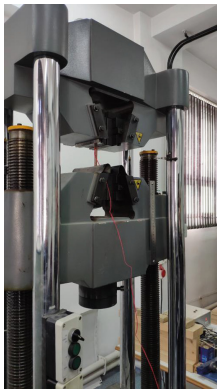
Fig. 2. Dumbbell sample fixed in the press
