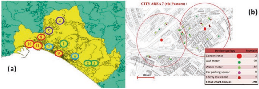
Fig. 2 (a) The 11 city areas in Salerno map; (b) in the zoomed view of area n.7, the position of concentrators and meters
