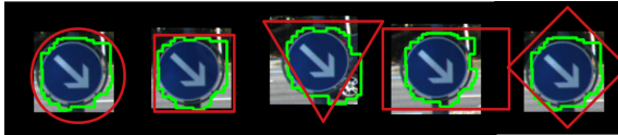
Fig. 6. Geometric shape association via contour comparison. Road sign shapes are generally simple geometric shapes such as circles, squares, triangles, and rectangles.
