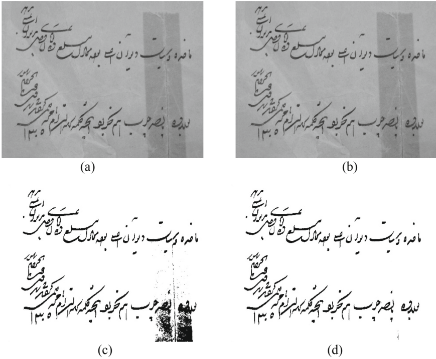
Fig. 6. (a) Median filtering image. (a) Gaussian filtering image. (b) The result of mean algorithm. (c) The result of the Otsu's algorithm. (d) The result of ours algorithm
