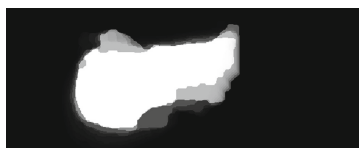
Fig. 4. Example of a MASH. Pixel intensities are correlated with the probability of the corresponding pixel to be selected as seed point for the corresponding slice.
