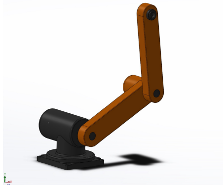
Fig. 2. 3D SOLIDWORK model of the 2-DOF robotic manipulator.
