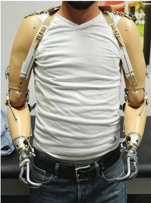
Fig. 4.5 Typical configuration of body-powered transhumeral prostheses for the bilateral amputee. Wrist rotation, wrist flexion, terminal device opening, and elbow flexion are controlled by a single control cable
