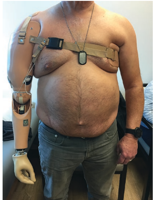
Fig. 4.1 Transhumeral hybrid prosthesis with dual-site myoelectric control of hand and cable-actuated body-powered control of elbow
