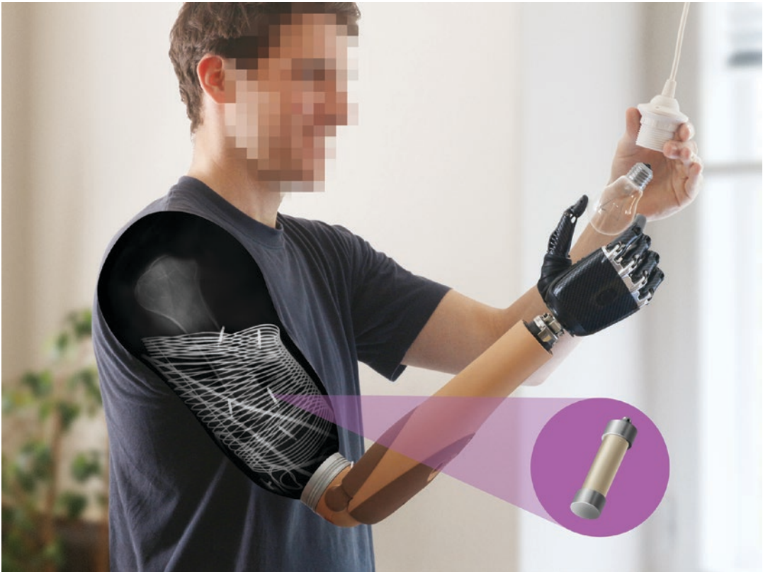
Fig. 14.1 A patient using the IMES system to handle a light bulb. An X-ray of the stump is shown, which includes the individual sensors of the system as well as the circumferential coil which is embedded into the prosthetic
