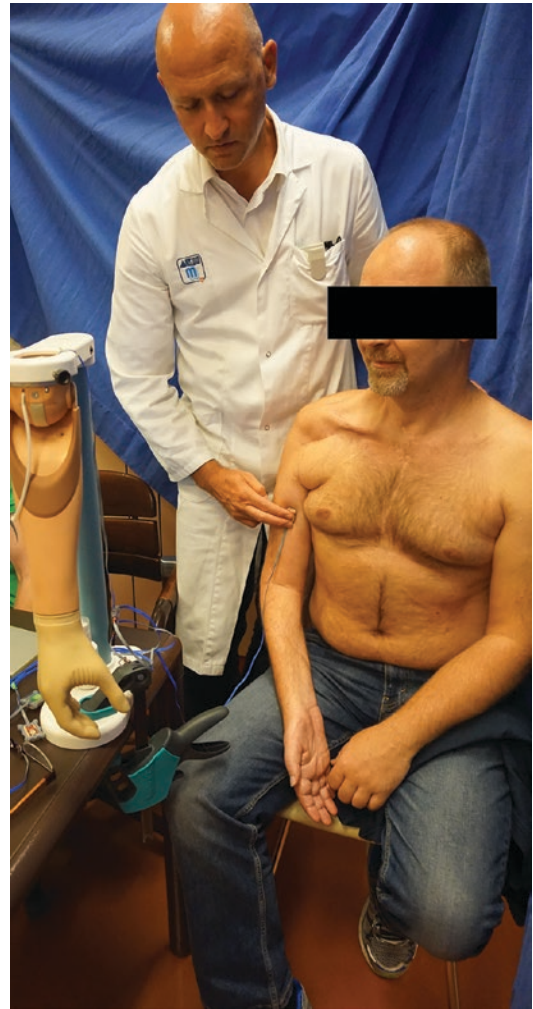
Fig. 17.1 Set-up of a table-top prosthesis. Transcutaneous electrodes are placed over muscles, where they sense and record EMG activity. (© Laura Hruby)
