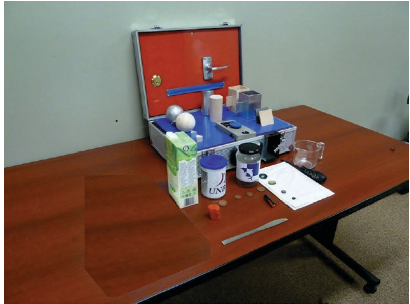
Fig. 7.4 The Southampton Hand Assessment Procedure (SHAP)—The complete set of tests based on activities of daily living are supplied in a single case. The test takes about 20 min to complete and provides a single number that measures the functional range for the hand. (c) Peter Kyberd
