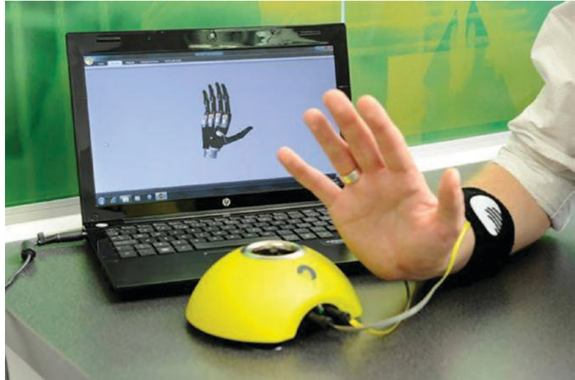
Fig. 20.2 Myoelectric site testing and training with virtu-limb from Össur Touch Solutions. (Used with permission from Össur Touch Solutions)
