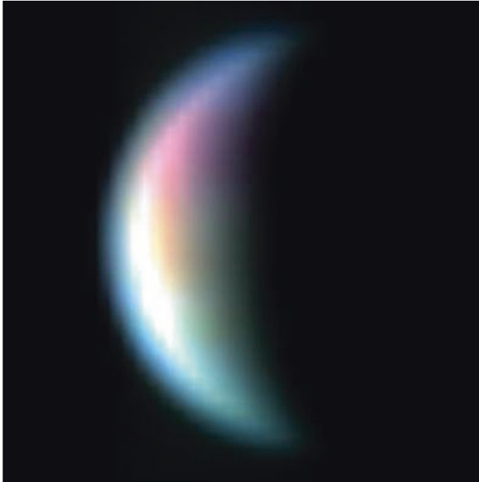
Fig. 7.4: Rosetta's VIRTIS instrument took this composite infrared view of the Moon on 4 March 2005, prior to closest approach to Earth, from a distance of 400,000 km. The spatial resolution is 100 km per pixel. It combines images at three different infrared wavelengths (2,225, 3,000 and 3,650 nanometers). Red represents the basaltic plains known as 'maria', while blue represents the ancient highlands. (ESA)
