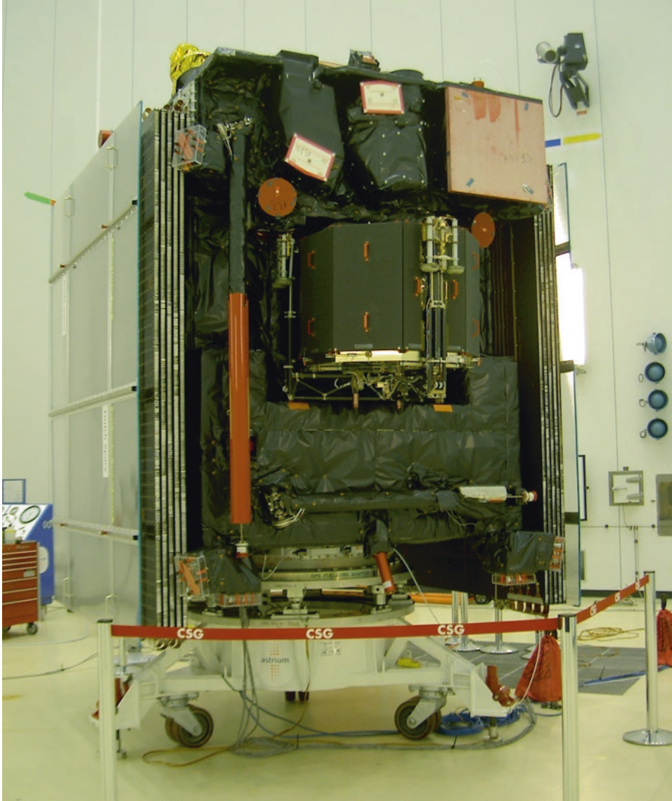
Fig. 6.7: The Rosetta orbiter and its lander (center) in the clean room at Kourou in January 2004. Note the folded solar arrays on either side of the orbiter. (ESA)
