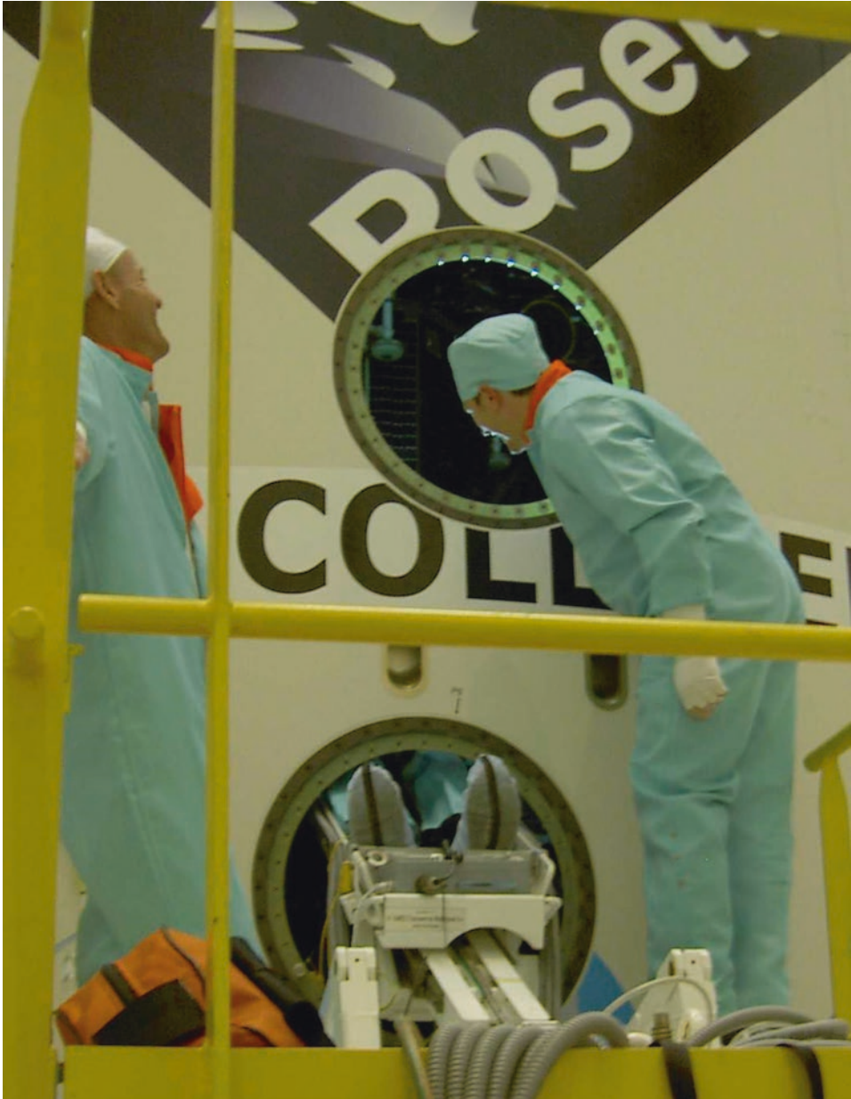
Fig. 6.11: A technician working inside the payload fairing to arm the lander's harpoons and remove their protective covers. (ESA)
