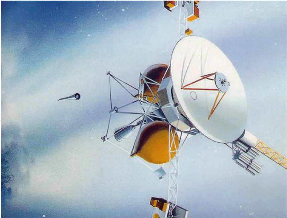
Fig. 3.3: NASA's Comet Rendezvous and Asteroid Fly-by (CRAF) mission was to be based on a new, nuclear-powered, Mariner Mark II spacecraft. It would make an asteroid fly-by en route to Comet Tempel 2, then fire an instrumented penetrator (left) into the nucleus and fly alongside the comet for three years, examining the formation of its coma and tails. (NASA)
