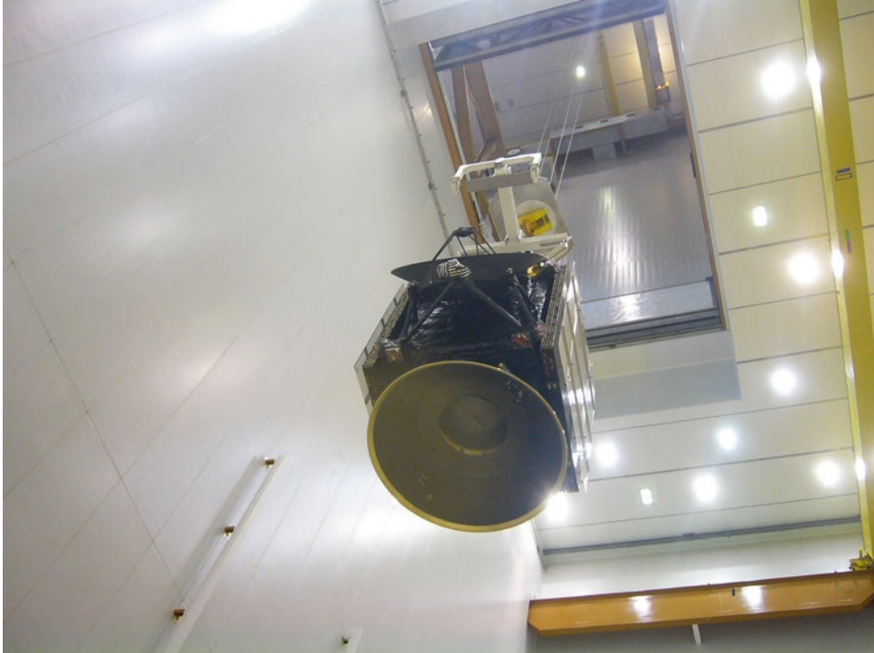
Fig. 6.8: On 16 February 2014, Rosetta and its payload adapter were lifted about 40 meters in the Final Assembly Building, ready for mating with its Ariane 5 launch vehicle. (ESA)
