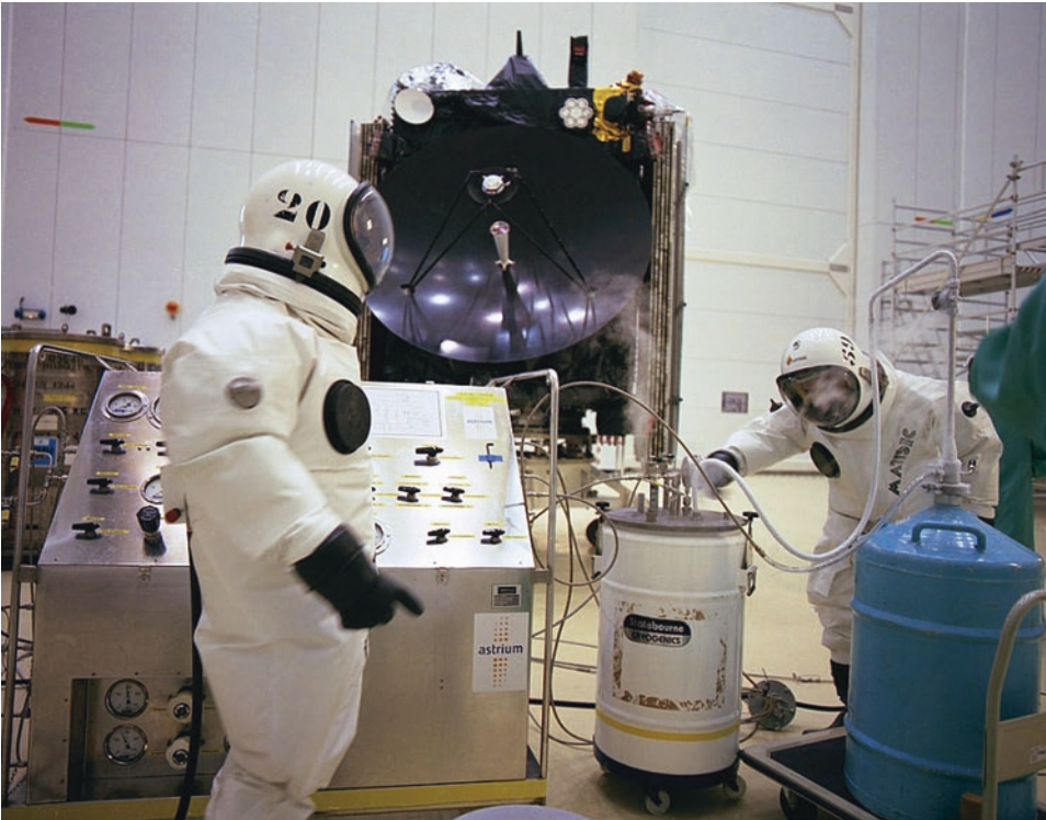
Fig. 6.6: MMH propellant being loaded into the Rosetta orbiter by a team from Astrium Ltd., on 27-28 January 2004. (ESA-CNES-Arianespace)
