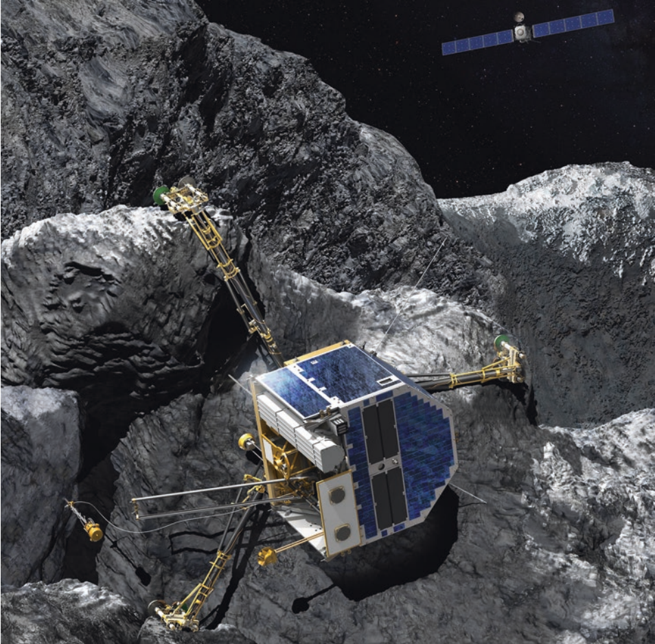
Fig. 9.11: A July 2015 artist's impression of Philae's final resting place, based on images provided by its ÇIVA camera system. Trapped in a hollow, it is lying on its side with only two of its three feet in contact with the ground. The rough terrain limits both its supply of solar energy and its communications with the Rosetta orbiter. (CNES/A. Torres; IAS/J-P. Bibring. Illustration D. Ducros)
