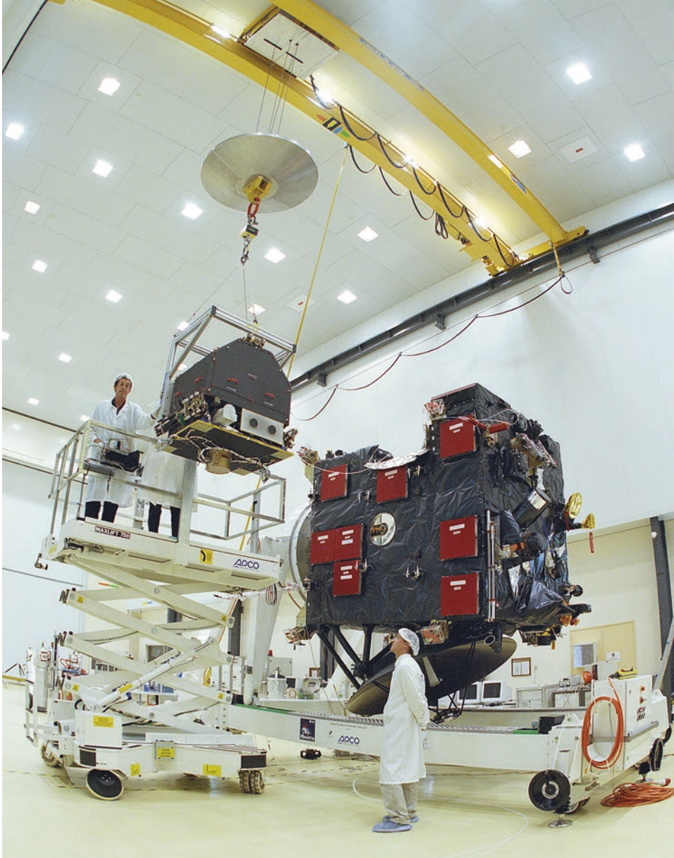
Fig. 4.9: The Rosetta spacecraft and the lander at the Center Spatial Guyanais (CSG) facilities in Kourou, French Guiana, in September 2002. The high-gain antenna is visible on the upper face, and instruments can be seen at the left. The solar arrays have yet to be attached. (ESA-Service Optique CSG)
