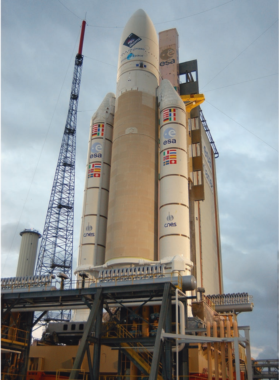
Fig. 5.15: The fully assembled Ariane 5G+ on the launch pad at Kourou on 1 March 2004, showing its core stage and twin solid-fueled boosters. (ESA-CGS-CNES-Arianespace)
