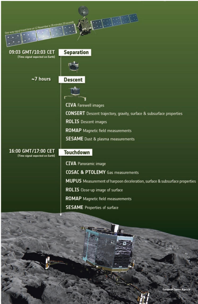
Fig. 9.6: The main scientific activities planned for Philae during its descent and touch-down. Timings are approximate. Confirmation of a successful touchdown was expected in a one-hour window centered on 16:02 GMT (CET was one hour ahead). The first image from the surface was expected about two hours later. (ESA-ATG Medialab)
