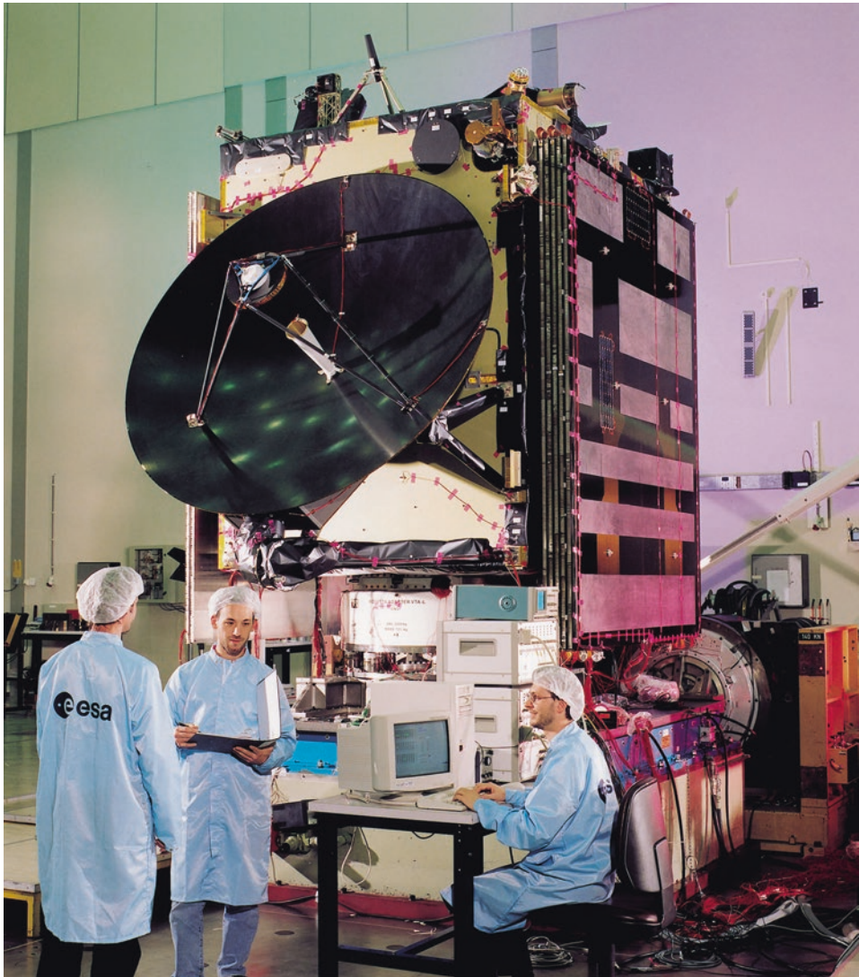
Fig. 4.6: The Rosetta structural and thermal model (STM) during vibration testing at ESTEC in January 2000. (ESA/A. Van Der Geest)
