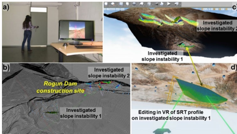
Fig. 5 Rogun site in virtual reality. a Researcher visiting the site in VR. b General semi-transparent surface view showing subsurface profiles. c Illuminating collected subsurface data near the Rogun site inside the virtual environment. d Visualisation of geophysical
