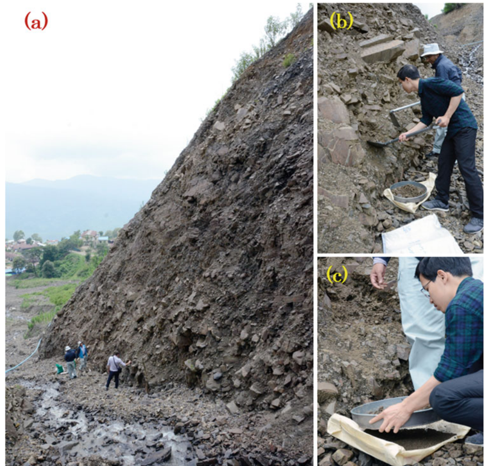
Fig. 6 Photos of soil sampling at a valley wall of the displaced landslide block. a Photo of sampling location from the top of gully, b Photo of sampling, c Sieving of sample
