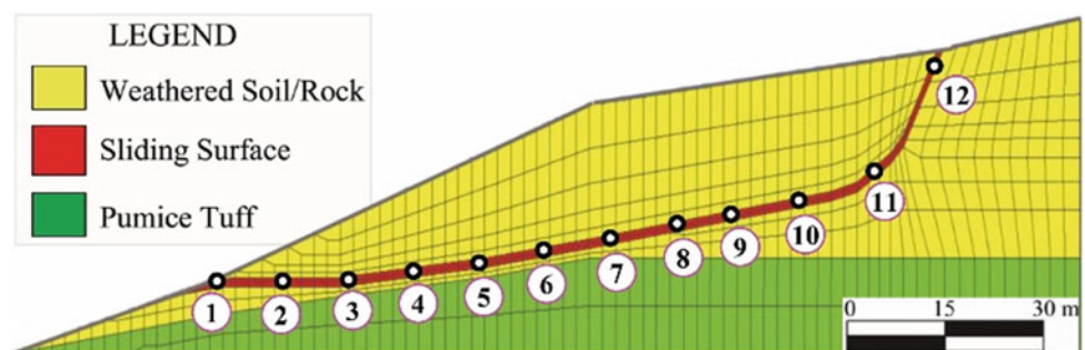
Fig. 9 Location of the observed point for measuring F_{s,local}
