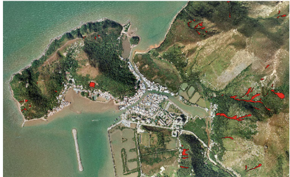
Fig. 3 Automatic identification of recent natural terrain landslides from aerial imageries
