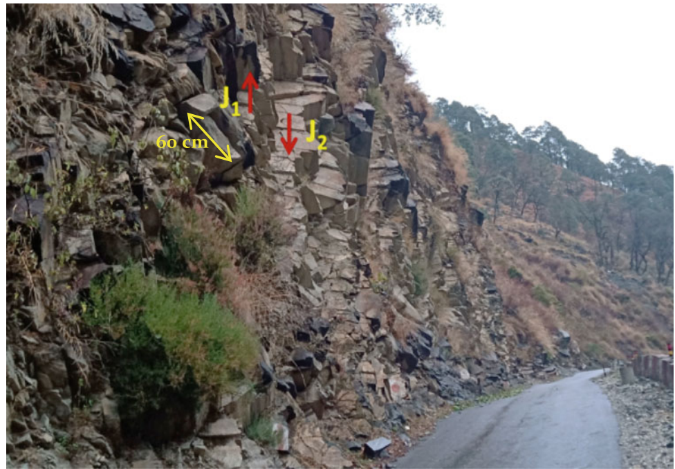
Fig. 8 Field photograph of the illustrated partially stable rock slope in the Higher Himalayas
