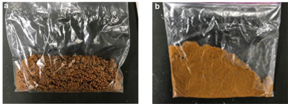
Fig. 5 a Natural condition of the Kpfa lower part-b (left), b Kpfa lower part-b crushed by wooden hammer (right) (sampled near sliding surface)
