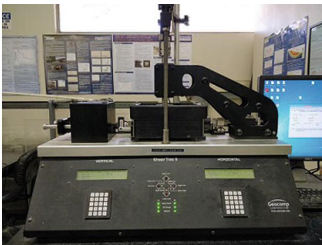
Fig. 1 Cyclic simple shear device used for this study
