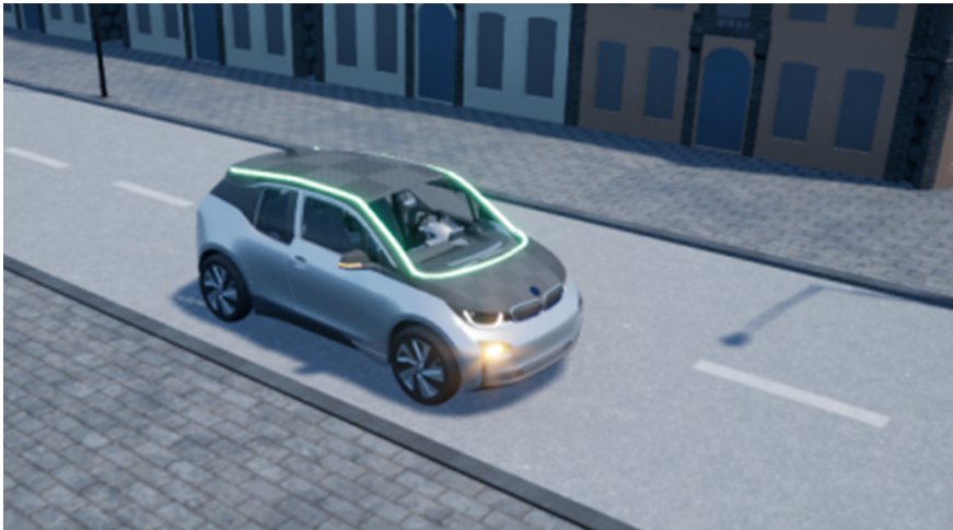
Fig. 1. External LED light-band on a CAV as eHMI used in the EU project interACT [6].
