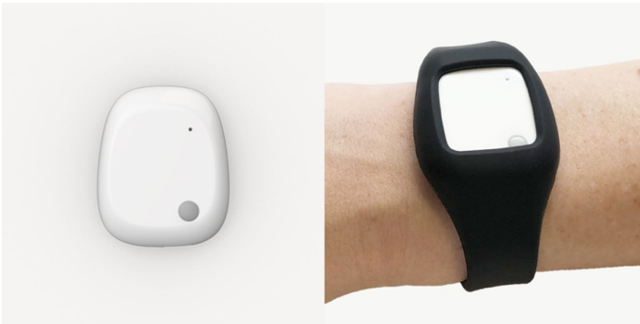
Fig. 1. (Left) Mble Labs MetaMotion R+wearable sensor, (Right) MetaMotion R+wearable sensor in the watch style silicone case.
