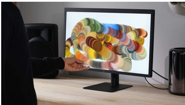
Fig. 2. Movement and gesture by the user is sent to the ABLE Music painting and music application to generate audio, visual and haptic feedback (through the sensor's vibration motor).
