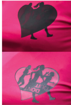
Fig. 2. Top image, thermochromic ink hiding the motivational message. Low image, thermochromic ink disappears revealing the quote “Don’t Quit, Do It”
