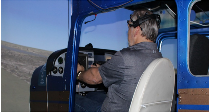
Fig. 1. Participant in the Cessna 172 simulator with the 14-channel wireless EMOTIV EPOC + EEG headset.
