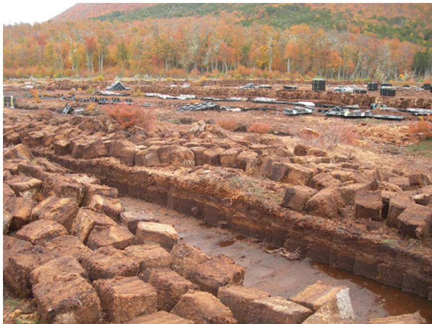
Fig. 7 Peat mining in a Sphagnum magellanicum bog from Tierra del Fuego. Peat is cut with shovels and is stored on “secaderos” in order to reduce its water content
