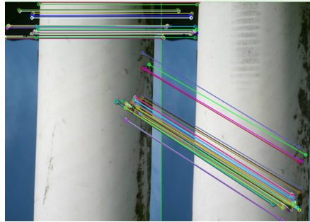
Fig. 2. The result of feature matching under parallax shows different homography.
