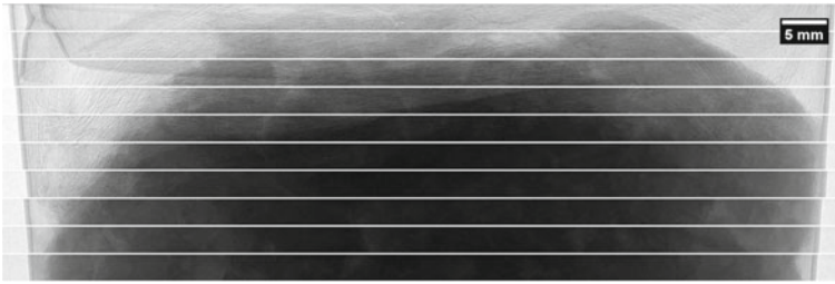
Fig. 5.12 Collage of a sample projection for each of the ten considered vertical stages. Due to the limited vertical size of the beam, the height of each projection consists in 51 pixels. The projections cannot be easily stitched together to compose a single projection of 510 pixels height because of the unknown angular shift and actual angular range covered induced by the continuous mode acquisition: the registration is performed within the reconstruction step
