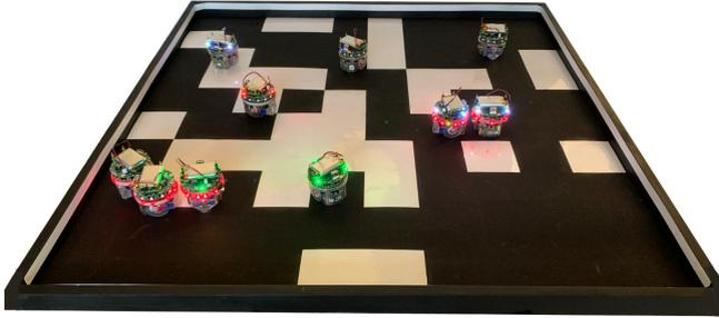
**Fig. 1.** The Pi-puck robots move in an  $1 \times 1 \text{ m}^2$  arena covered by 68 black and 32 white tiles. The robots’ goal is to determine the fraction of white tiles by using their ground sensors. A part of the swarm act as Byzantine robots that disseminate wrong estimates. Using their LEDs, the robots communicate events—such as the receipt of a new block or the receipt of the consensus signal—to the experimenter for visual analysis.
