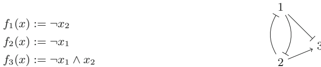
Fig. 1. Example of Boolean network f and its influence graph G(f) where positive edges are with normal tip and negative edges are with bar tip.
