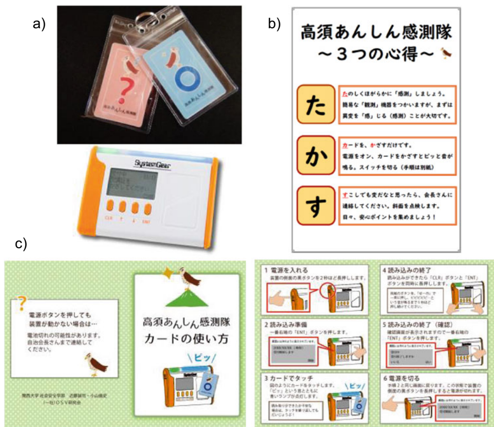
Fig. 7 a IC cards printed “normal” and “abnormal” and IC card reader, b “Takasu voluntary slope observation team -three hints” and c a card reader handling manual
