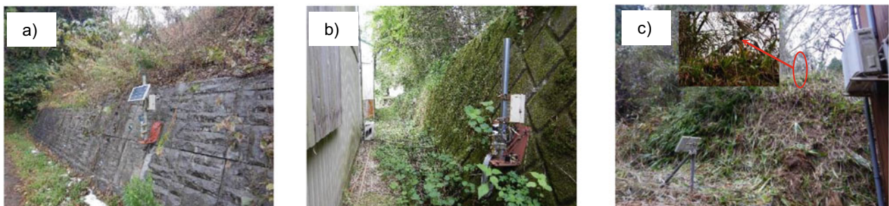
Fig. 6 Slope measurement/monitoring using POCKET, a block retaining walls along farm roads, b block retaining walls behind elementary school gymnasiums, and c slopes behind houses
