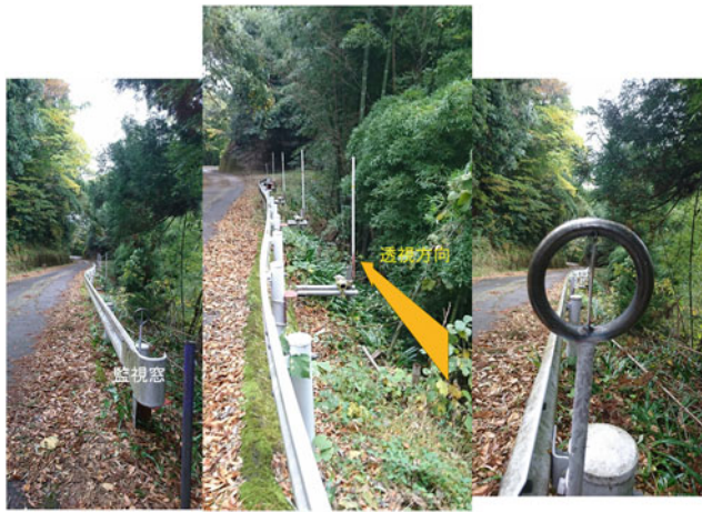
Fig. 3 “See-through poles” using observation poles and reference pole with a viewing window
