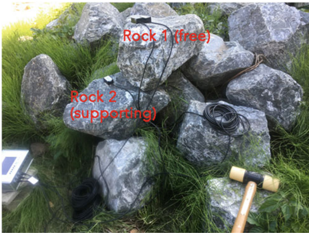
Fig. 3 The first configuration of mound of rocks. Another rock will be leaned on Rock 1 for the second test condition
