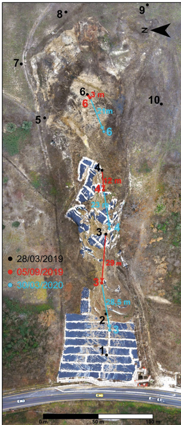
Fig. 12 Example of vectors of horizontal displacements obtained from GPS data for the range periods 28.03.2019–05.09.2019 (red vectors) and 05.09.2019–30.03.2020 (light blue vectors)
