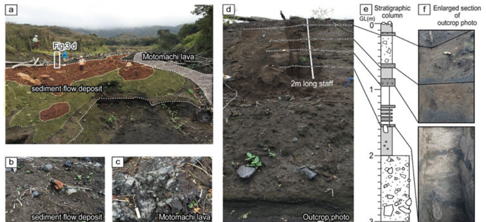
Fig. 3 Condition of sedimentation and geological profile in the downstream area of the survey site (Okanazawa) in Izu-Oshima (JSCE 2015)
