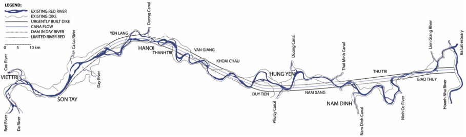
Fig. 6. To canalize the Red River was proposed by Nguyen Canh in 1920s, aiming to improve the ability of water discharge to the East Sea in the rainy season. (Pham 2010, redrawn from [13]).
