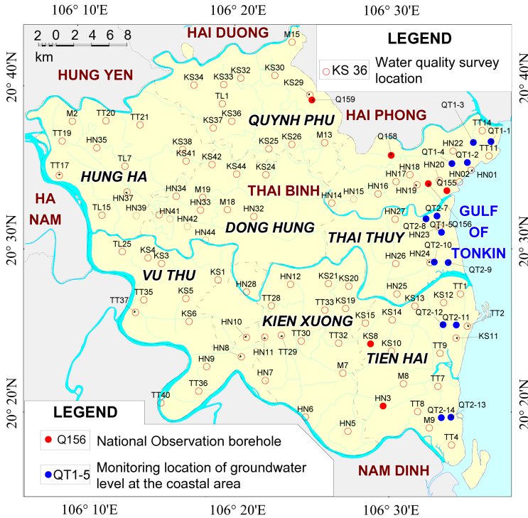
Fig. 4. Map showing the sampling locations for groundwater of Holocene aquifer, in situ measurements and monitoring the groundwater level in coastal area
