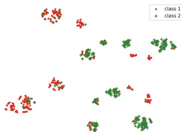
Fig. 1. An example of credit dataset visualization. Normalize the digitized data features to [0,1] and use t-SNE to visualize the data. Data is reduced to 2- D space. The dataset has two classes (1 and 2) and multiple data-dense divisions of each class.
