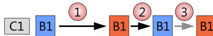
Fig. 4. Component C_1 from Fig. 3 performing two small steps in order to reach C_0 's larger time step. First, C_1 performs its initial step and writes its computed items into its associated target buffer (1). Afterwards, C_1 is applied again and performs the next step. In this case, C_1 reads its source values from the originally intended target buffer and writes into its original source buffer (2). To ensure that the finally written values will end up in the correct target buffer , we have to copy the updated items from the source into the target after execution of the second step (3).
