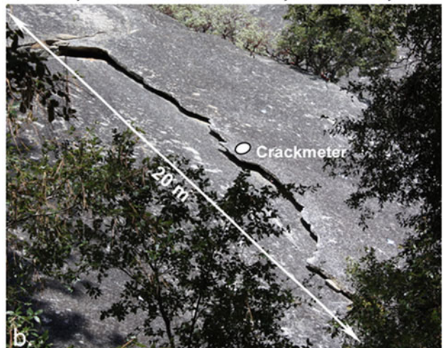
Fig. 29 a Monthly maximum aperture of the rock sheet in b showing the seasonal cycles and drift indicating the extension of the sheet (after Collins and Stock, 2016)
