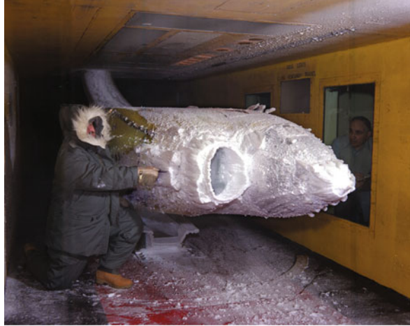
Fig. 15.5 Icing tunnel tests on the NASA Lewis research center. Tests of a reduced model of a commuter aircraft. Source: NASA
