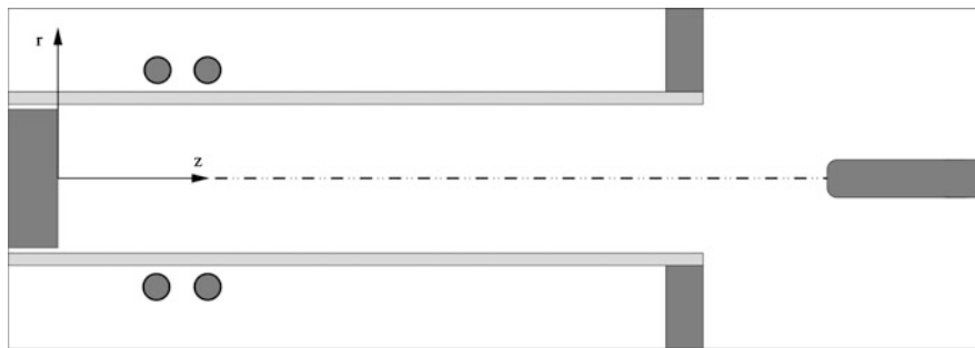
Fig. 16.10 Inductive plasma wind tunnel: torch, coil, and probe (Credit: T. Magin [27])
