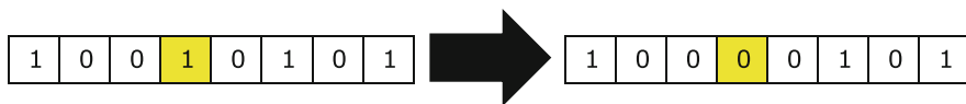
Fig. 8.6 Example of bit switching mutation. A random point on the chromosome of an individual value is changed
