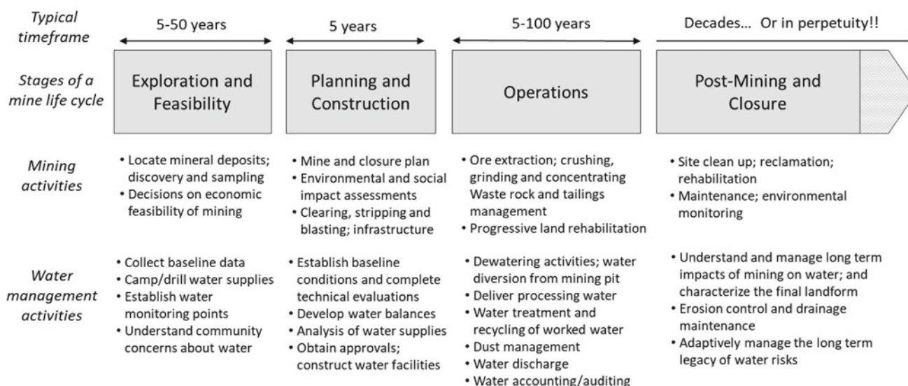
Fig. 21.1 Typical stages in the life cycle of a mining operation, and the associated water management activities; modified from (Government of Canada 2017; Department of Industry, Science, Energy and Resources 2016)
