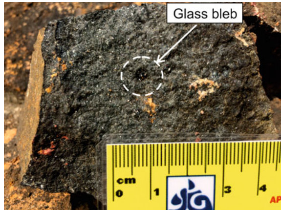
Fig. 30 Basalt sample with a glassy bleb in it (pointed by arrow)
