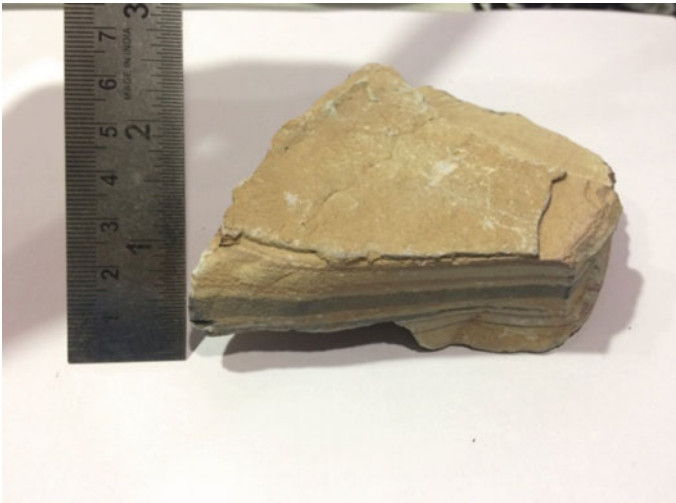
Fig. 27 Thinly laminated shale sample, Vahalwadi
