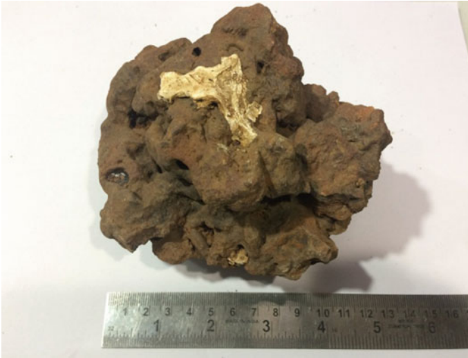
Fig. 33 Secondary laterite sample, Sarjekot
