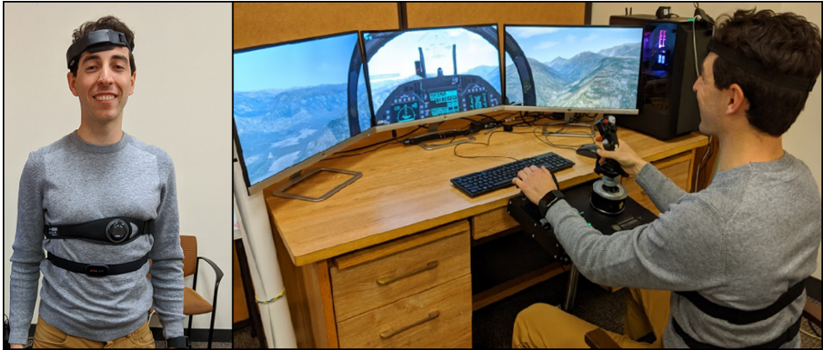
Fig. 2. Sensor configuration (left) and testbed environment with desk mounted Tobii Eye Tracker (right).
