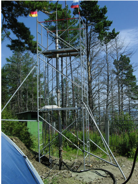
Fig. 1 The Borehole Generator of Seismic Waves (BGSW) mounted at one of the sides of the Angarskiy fault
