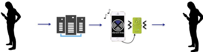
Fig. 2. This image shows the system used for all iterations of Vibrant Lives . Users connect to our custom server via our wireless network. Their data output is then captured and sent back to their mobile device using our mobile phone application. The mobile phone application creates a data sonification, which is transformed into vibrotactile stimulation using the tactile transducer.
