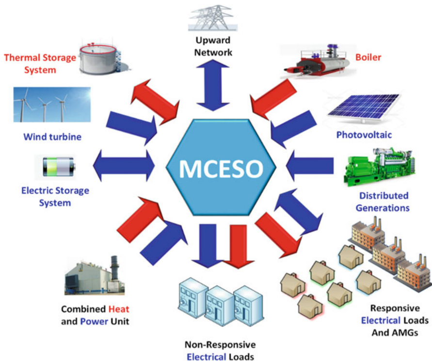
Fig. 11.1 The diagram of MCESO energy interactions
