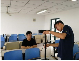
Fig. 4. Data collection process. The horizontal distance between the Kinect camera and a student was 120 cm
