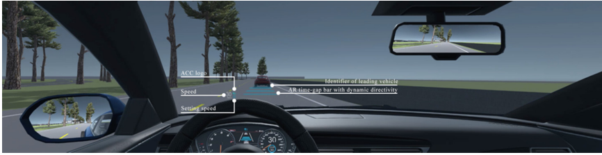
Fig. 4. HUD-HMI2 (the AR time-bar dynamically points to the leading vehicle).
