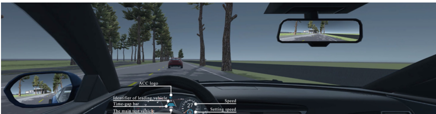
Fig. 2. Dashboard-HMI (baseline HMI that design elements are displayed only on the dashboard).
