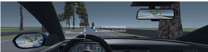
Fig. 3. HUD-HMI1 (the AR time-gap bar is relatively stationary with the main test vehicle).
