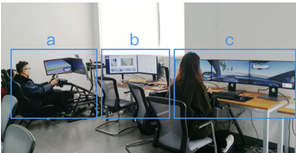
Fig. 1. Experimental Equipment (a is the main test vehicle, c is the auxiliary test vehicle, and b is SCADA).
