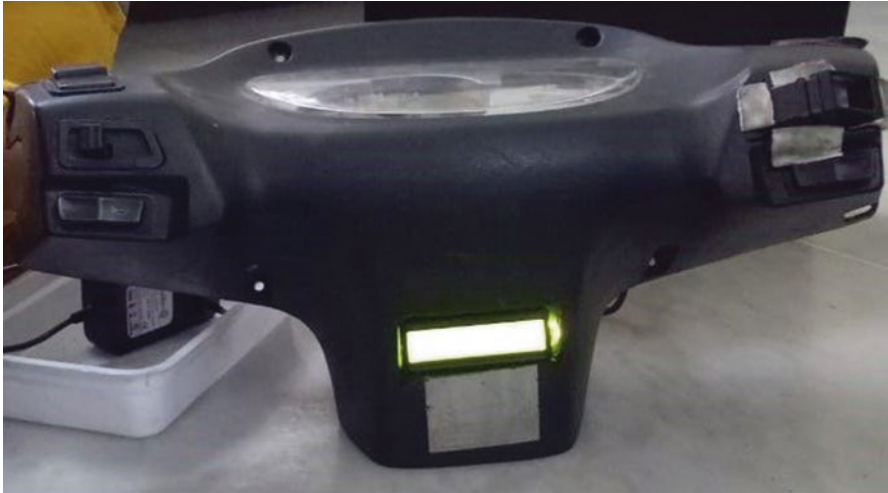
Fig. 9 Prototype model of the proposed system for fingerprint scanning and display of result
