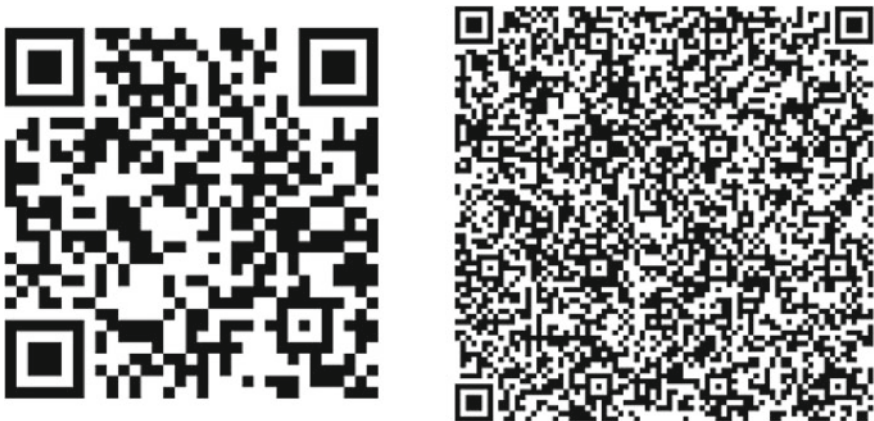
Fig. 2.5 QR-representations. Left: the author's name and title. Right: the author's name and title, along with his degrees and mailing address. The finer the (binary) detail in a QR, the more information is stored in it and, the finer the detail, the higher the spatial complexity
