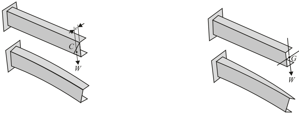
(a) Bending of channel section without twisting, when the load W acts through the shear centre C .
