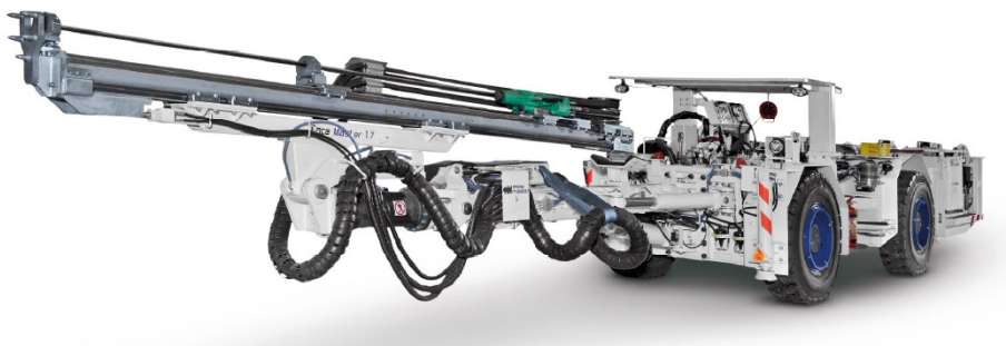
Fig. 2. Self-propelled drilling and anchoring vehicle Face Master 1.7 [13].
