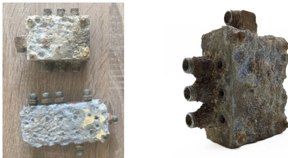
Fig. 5. Grease distributors after the service life.
