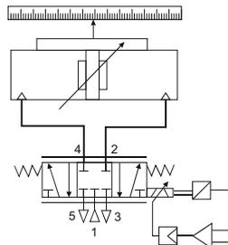
**Fig. 3.** Electro-pneumatic servo-drive diagram with rodless cylinder.
