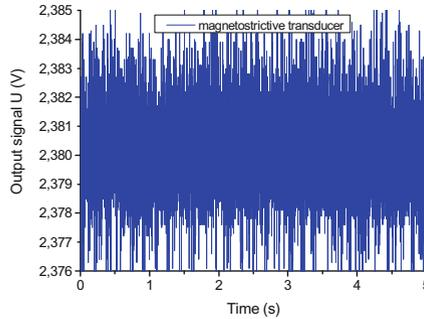
**Fig. 6.** Measurement noise of the BTL5-A11-M0600-P-S32 position transducer.
