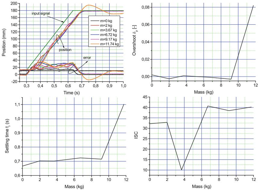
**Fig. 9.** Tracking control with variable load mass
