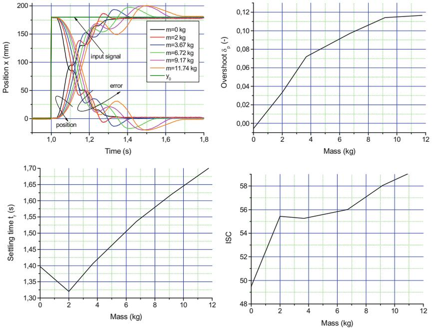
**Fig. 8.** Changeover control with variable load mass.
