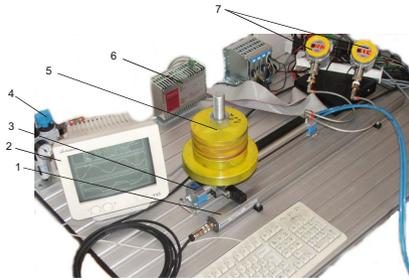
**Fig. 7.** A general view of the test stand: 1 – position transducer, 2 – screen, 3 – rodless cylinder, 4 – FRL unit, 5 – mass load, 6 – power supply, 7 – pressure transducer.
