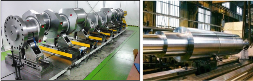
Fig. 3. Machining of a monolithic shaft of a marine engine and final product of the machine driveshaft (photo FPD)
