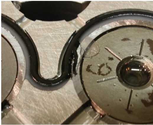
Fig. 2. Seal defective due to excessive temperature rise [19].
