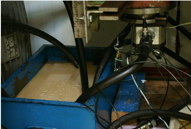
Fig. 4. Stand for testing gear pumps in low temperature chamber
