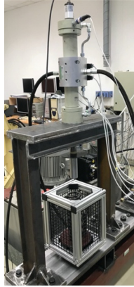
Fig. 1. Test rig with the integrated hydraulic actuator for spring stiffness measurement.
