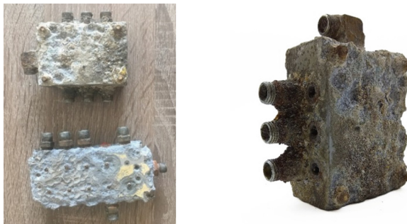
Fig. 5. Grease distributors after the service life.
