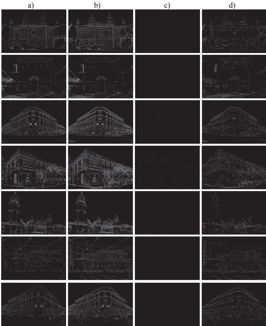
Fig. 18. Rows: a) Canny using Sobel 3 \times 3 , b) Canny using proposed A 3 \times 3 , c) Edge pixels found only by a, d) Edge pixels found only by b
