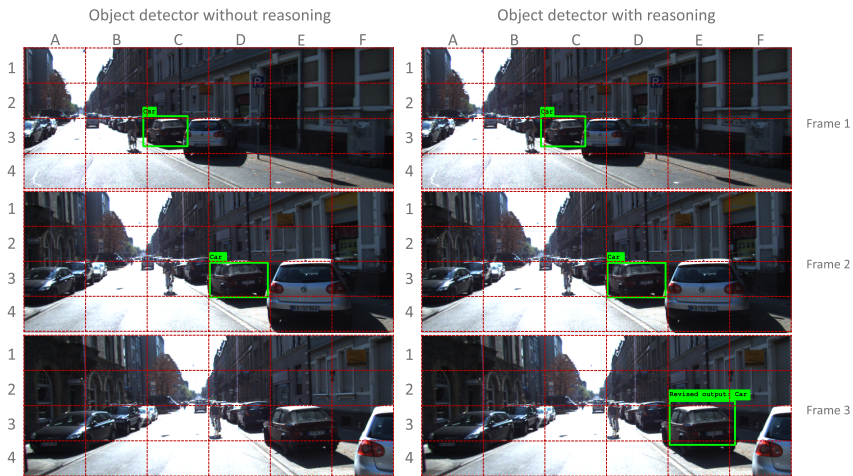
Fig. 3. Left: an object detector recognizing the object of interest in the first two frames but missing the object in the third frame. Right: revised output at frame three after the application of spatial reasoning in addition to the object detector.
