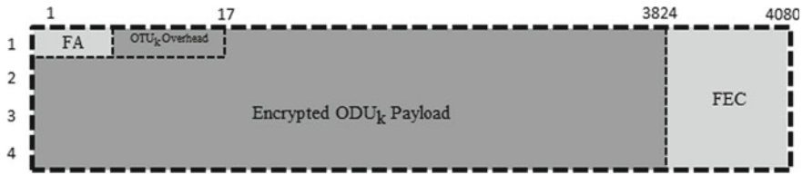
Fig. 9 The Structure of the OTN 10/100 Gb/s frame with encrypted ODU
