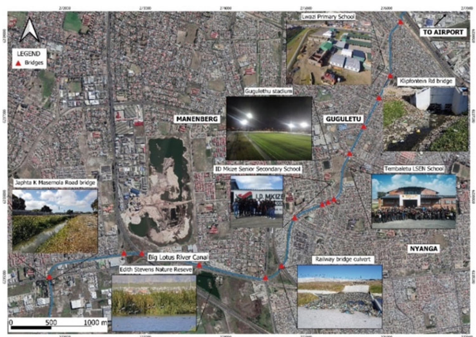
Fig. 3 The Great Lotus Canal (or BLC in Fig. 2; blue line with red triangle markers) collects stormwater from the Cape Town airport and its industrial area (upper right) and transports it to the north-western corner of the PHA (lower left), where—just outside of the image edge—it is intercepted during low-flow periods by a weir connected to a main sewage line
