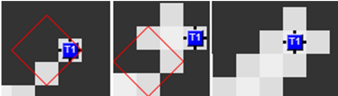
Fig. 8. The agent utilizes clear actions to break out of a contained space. The agent clears the obstacles that are most likely to open it up to free space.
