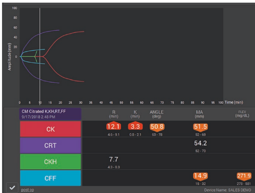
Fig. 21.7 New to the TEG system technology is the measurement of clot viscoelasticity using a resonance method. To measure the clot strength with the resonance method, the sample is exposed to a fixed vibration frequency. With LED illumination, a detector measures up/down motion of the blood meniscus. The frequency leading to resonance is identified and then converted to the TEG system readout. Stronger clots have higher resonant frequencies and higher TEG readouts. (With permission from Haemonetics Corporation)
