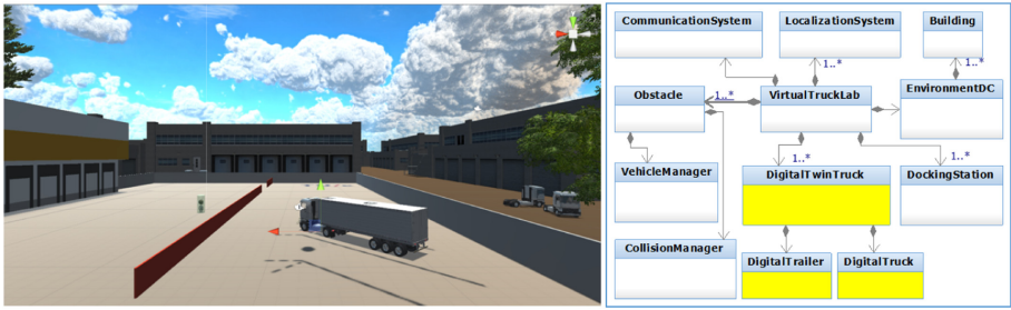
Fig. 2. Left, the 3D representation of the Truck Lab, including all the 3D assets: the buildings, the docking stations, the parking area, the obstacles inside the distribution center and the digital twin truck. Right, the high level components of the Virtual Truck Lab’s architecture containing: the virtual Truck lab, the digital twin truck with its truck trailer combination, the truck manager, the collision manager.
