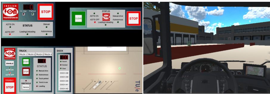
Fig. 6. Left, a GUI used: to monitor the truck's state, to select a docking station and monitor its state, to select a parking destination for the truck. Right, cabin camera view showing the environment from the driver's perspective.
