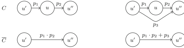
Fig. 2. Removing a vertex u . The vertex u' is a predecessor of u and u'' is one of its successors. The left side shows the changes when there is no edge from u' to u'' and the right side shows the other case, where (u', u'') \in E . Edge labels are \delta values.
