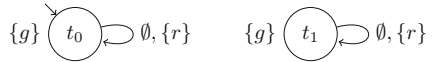
Fig. 2. A transition system over I = \{r\} and O = \{g\} that is not a model of \varphi_1 .
