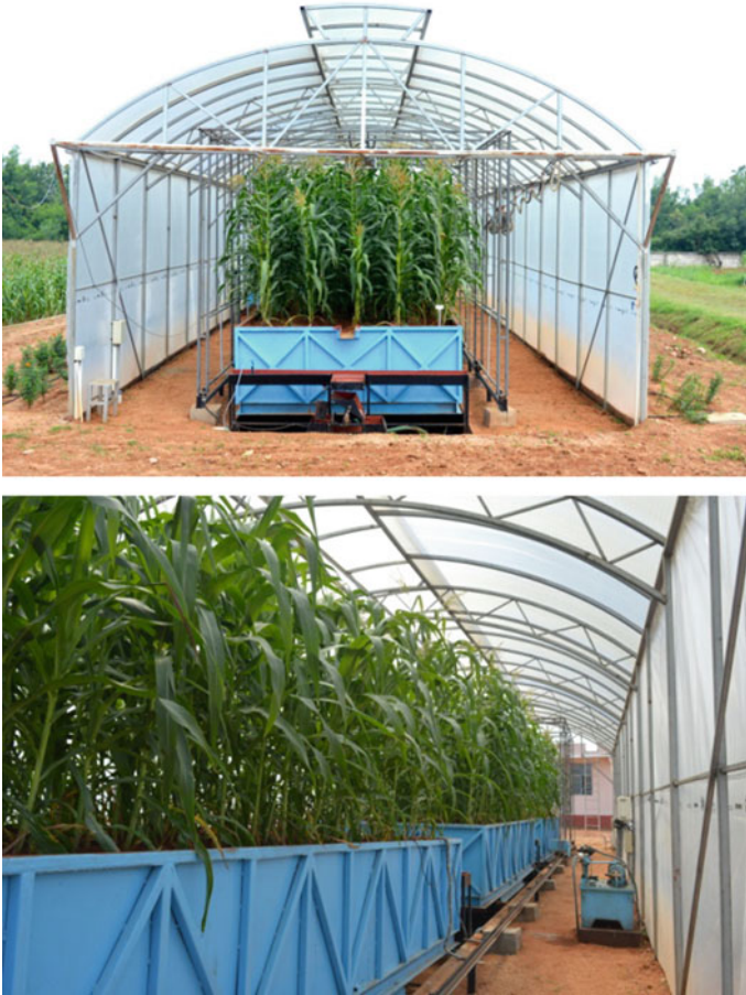
Fig. 30.2 Rainfall simulator system with soil bins and maize as a test crop
