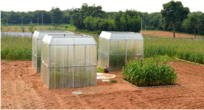
Fig. 30.4 Open-top climate chambers with maize as test crop
