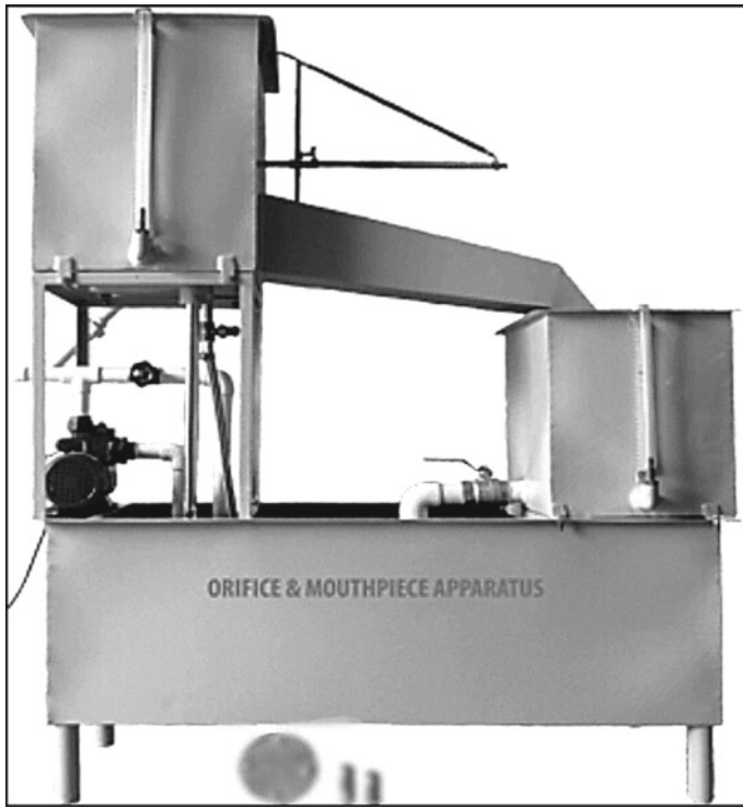
Fig. 15.7 Experimental setup of orifice apparatus
