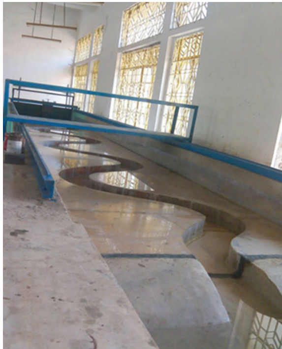
Fig. 16.6 Plain-metric view of experimental setup for the meandering channel
